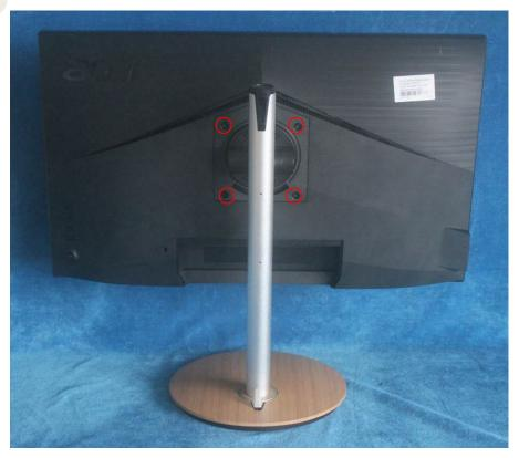
Remove the rear cover. Use a tool (like picture using) to open all latches. (Be careful the position of the key S2 board.)
